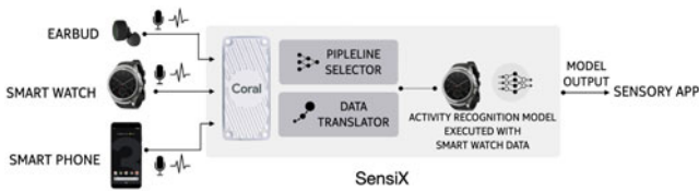
Fig. 1. SensiX stays between sensors and models and applies translation and selection operators to selectively choose the execution path for best-effort inference. Here, SensiX uses watch data and respective model to guarantee the best accuracy based on the outcome of the operators.
